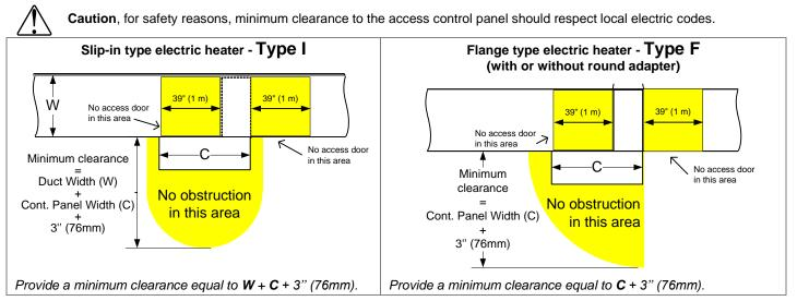
**Caution**, **Risk of electric shock and burns.** A minimum distance of 39" (1m) must be maintained between heating section and any opening or access door in the duct. This applies to all types of heaters. If such distance cannot be maintained, a protective guard (**C22.2 No.155 section 4.1.8**) must be installed to protect personnel from contact to heating elements and bare live parts.
